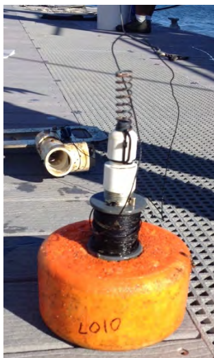
Figure 11 (left): A spring attachment design that interfered with the line spool release and was abandoned.
