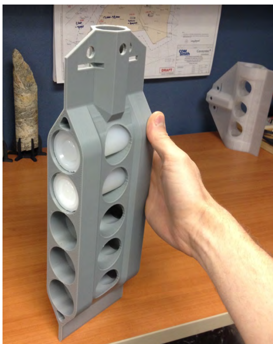
Figure 22: Prototype sampler frame to deploy cylindrical samplers to assess metal contamination in sediments, designed by Geosyntec (photo courtesy of Geosyntec).
